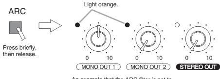
An example that the ARC filter is set to the MONO OUT 1 and MONO OUT 2 channels.
