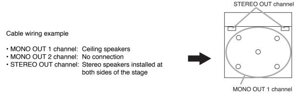
Step 1. Set the ARC filter only to the MONO OUT 1 channel (ceiling speakers).
