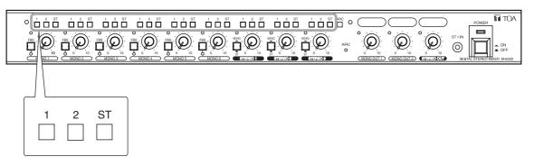
Pressing the Assignment switch "1" routes the input signal to the MONO OUT 1 output, switch "2" to the MONO OUT 2 output, and switch "ST" to the STEREO OUT output. Input signals assigned to the same output destination are mixed.
